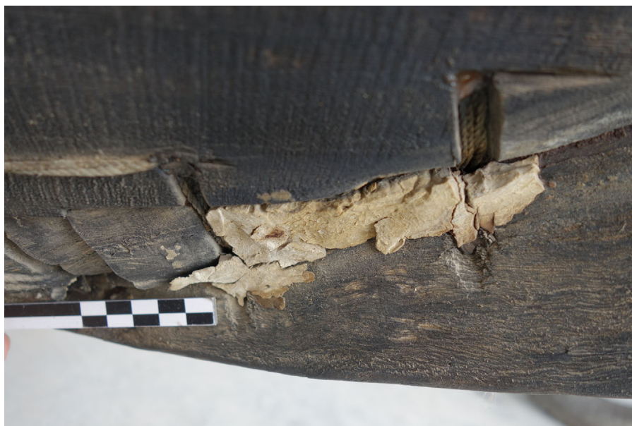
Figure 22. A white putty-like substance within the stitching fastening the outer post to the planking of kettuvallam B. (Image: Chiara Zazzaro).
