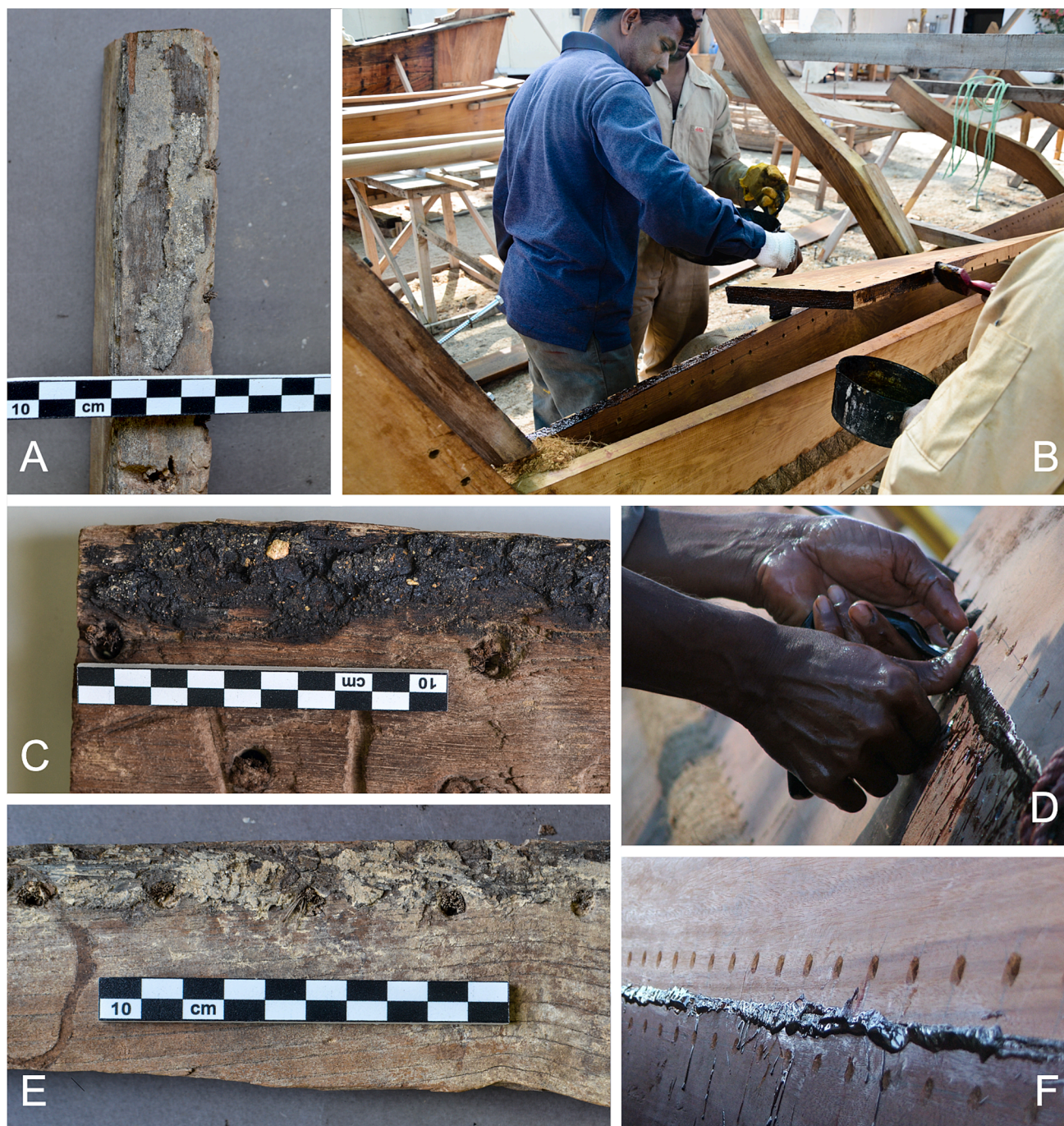
Fig. 5. (A): “Bitumen” on the edge of timber BA1104065.454 suggesting the practice of luting the seams of the planks before their fitting. (B): The luting process, in this case carried out using dammar resin, during the construction of the al-Hariri Boat, a reconstruction of a 13th century Indian Ocean sewn merchant vessel based on the illustrations of the Maqamat al-Hariri . (C-E): A thick layer of “bitumen” covers the section between the sewing holes and the plank’s edge on timbers BA0604145.175 and BA1104065.454. (D-E): The boatbuilders of the Jewel of Muscat , a reconstruction of a 9th century sewn cargo vessel based on the Belitung shipwreck discovered in Indonesia, used dammar resin to seal the seams of the planks after their fitting and before commencing the sewing. (Photos: A. Ghidoni).
