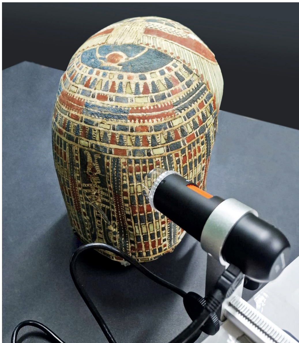
Fig. 5: Cartonnage discovered in tomb AGH026 scrutinized with a 5 Mpixels sensor-USB microscope equipped with a includable/excludable polarizing filter © EIMAWA.
