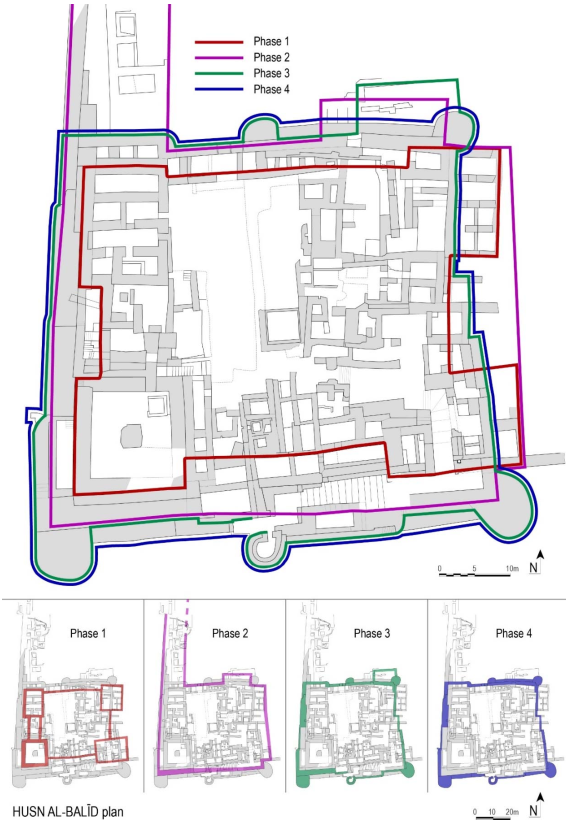
Fig. 37 - Plans related to the four different main constructional phases of the citadel (Plans by C. Passaro).
