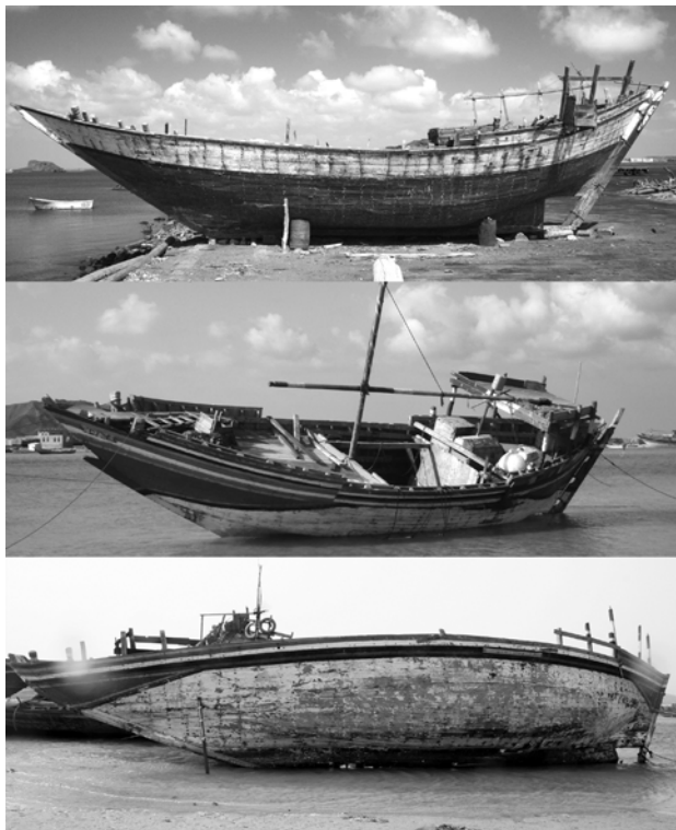
FIGURE 5. Three types of double-ended sanbūq found in Yemen — the ʿobrī (top) in Aden, and the zārūq (centre) and zāʿīmah (bottom), in Ghurayrah (MARES/J.P. Cooper, C. Zazzaro).
