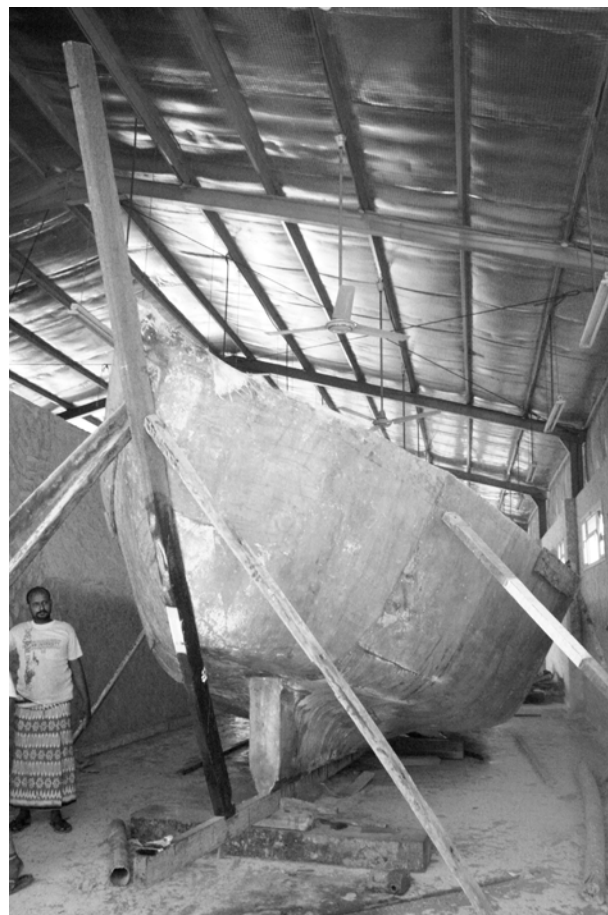
FIGURE 9. A fiberglass galbah under construction at al-Salīf. The hull form retains that of the wooden °obrī (MARES/J.P. Cooper).
