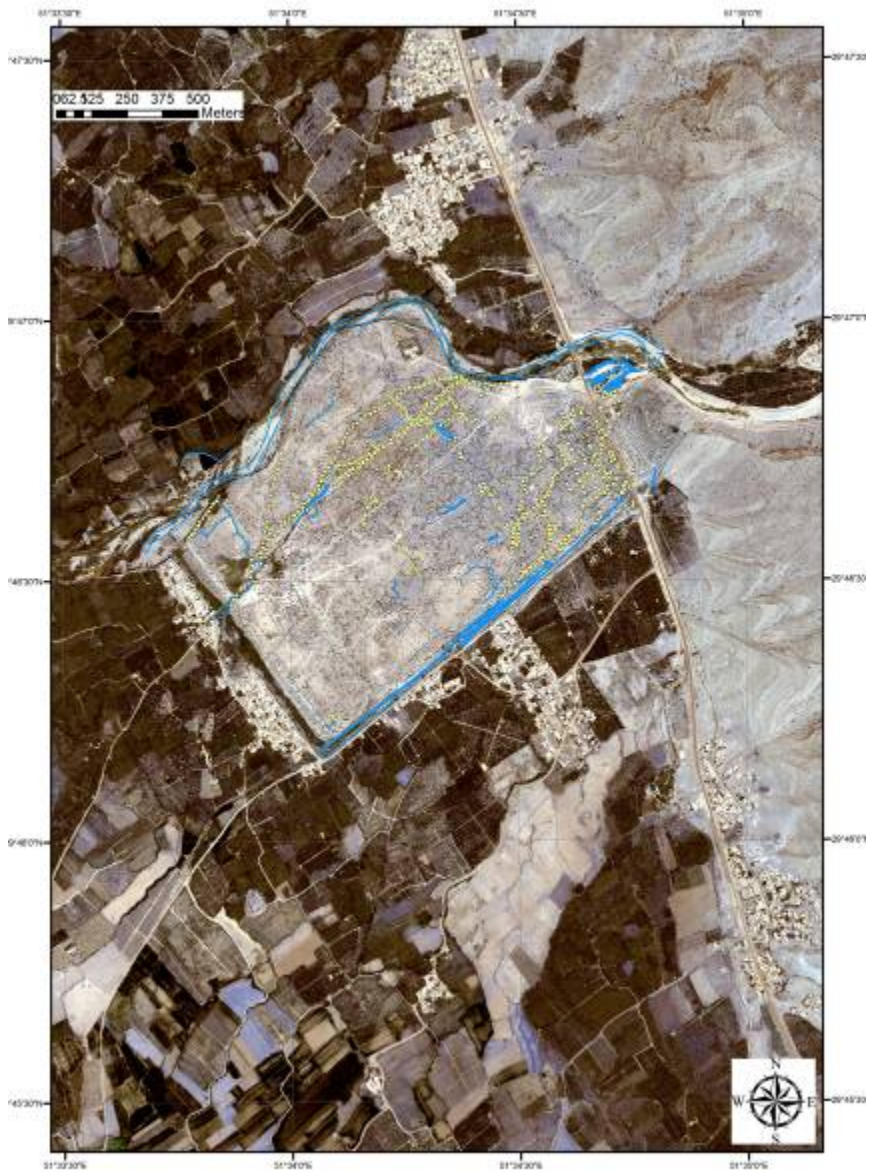
Fig. 45 - Digital cartography geo-referenced of the landscape around Bīšāpūr to scale 1:500; are visible the qanats (yellow layer) and the water places (blue layer) like river and artificial canals. Image modify by E. Cocca, after AUTOCAD map from CRS (Bīšāpūr of Research Center)
