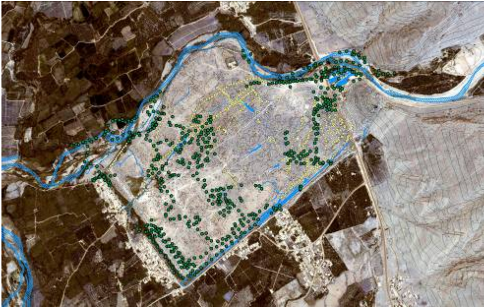
Fig. 46 - Localization Control Point for geo-referencing vector layer. Image modify by E. Cocca, after AUTOCAD map from CRS (Bīšāpūr of Research Center)
