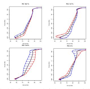
Figure 3. The effects on the mean aircraft trajectory (solid curve) of adding (red curves) and substracting (blue curves) a multiple of each of the first four principal components.
