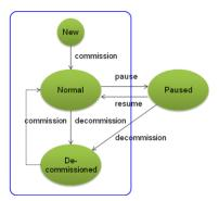
Figure 1. State transition diagram for a data node.
