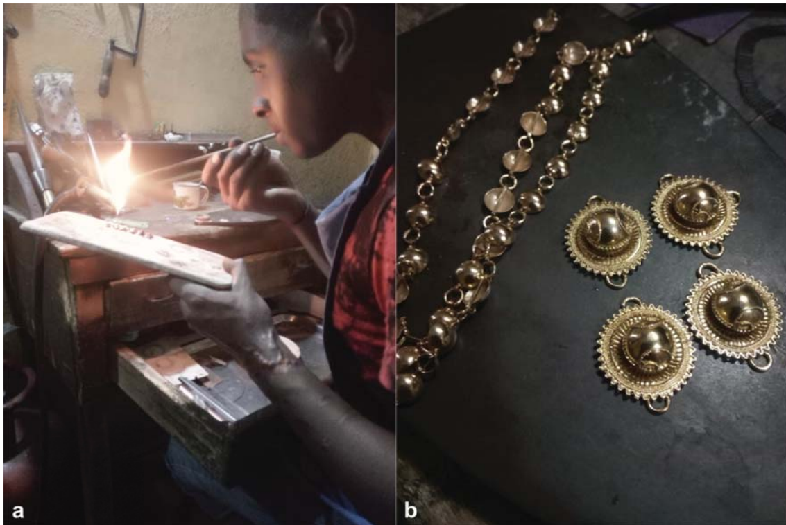
Fig. 9 - a) The goldsmith welds with menafia and torch; b) Gold chain and pendants with the traditional decoration called chat
