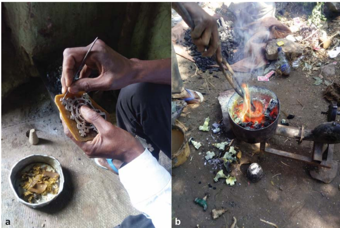
Fig. 8 - a) The craftsman draws the shape of the cross on a sheet of wax with the mekereti ; b) The melting with the use of kawri and forgia
