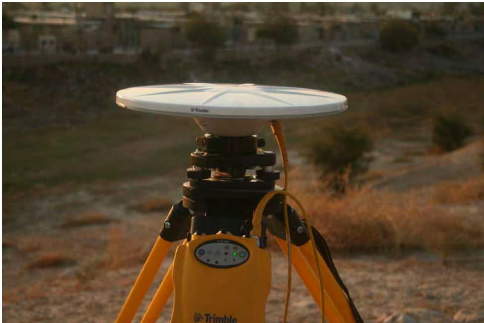
Fig. 10 - GPS base Trimble 5700/5800, after MAI
