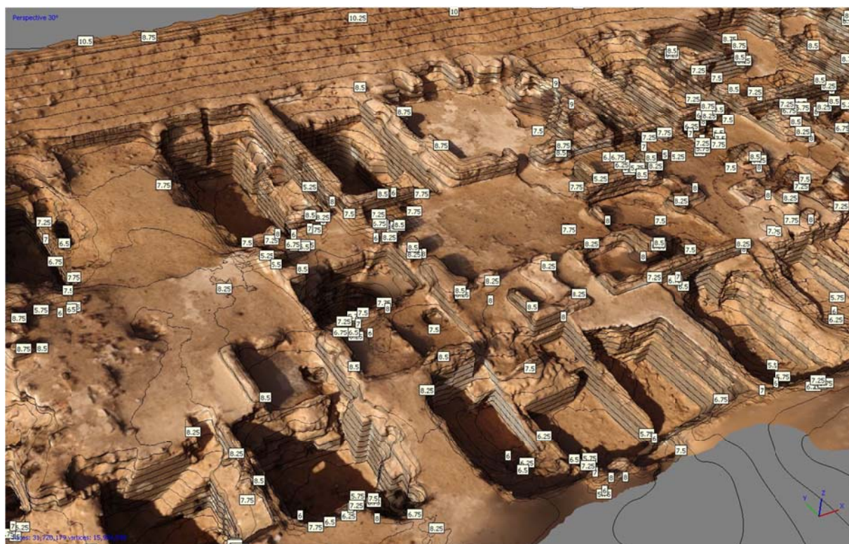
Fig. 3 - The 3D model of the North area after applying the tool to create contour polylines. The labels indicate the elevation each 25cm
